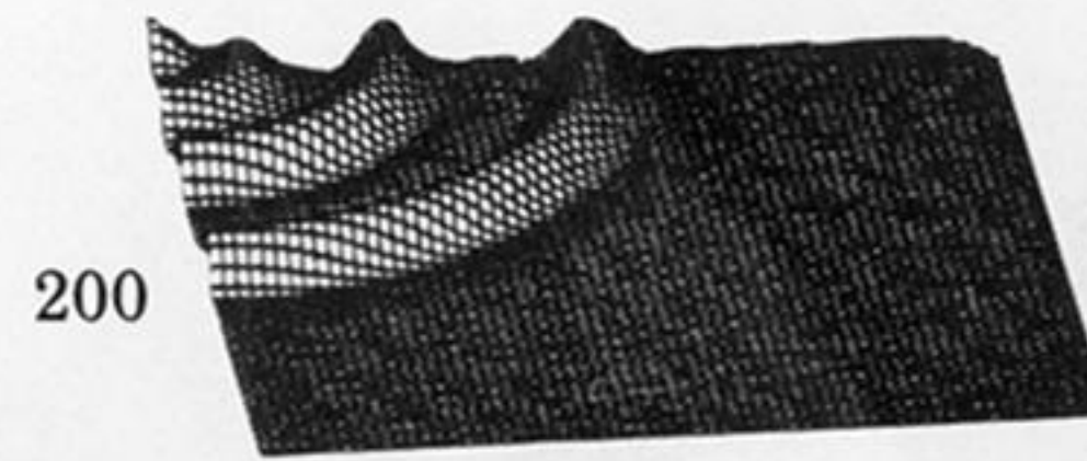
FIGURE 1. Time evolution of one quadrant of the two-dimensional intensity profile as the beam switches from a low to a high transmission state of the bistable system. The numbers indicate the resonator pass. The nonlinearity is saturable as in (1) with kL = 0.2 , F = 100 and input peak intensity |a(0,0)|^2 = 0.0375 . These parameters are explicitly defined by McLaughlin et al. (1983).
