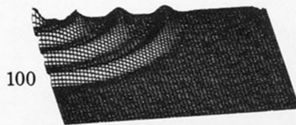
FIGURE 1. Time evolution of one quadrant of the two-dimensional intensity profile as the beam switches from a low to a high transmission state of the bistable system. The numbers indicate the resonator pass. The nonlinearity is saturable as in (1) with kL = 0.2 , F = 100 and input peak intensity |a(0,0)|^2 = 0.0375 . These parameters are explicitly defined by McLaughlin et al. (1983).
